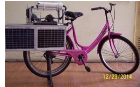
Bicycle-mounted, RO / UF unit operated with hybrid power system
